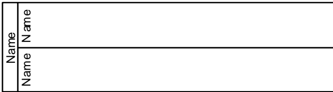
Figure 10.124 - Two Lanes in a horizontal Pool
