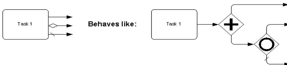
Figure 13.1 - Behavior of multiple outgoing Sequence Flows of an Activity
