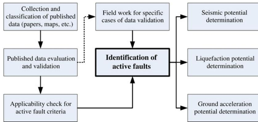
**Fig. 2** Procedure flow diagram for the characterization of active faults (Pavlidis et al. 2009)
