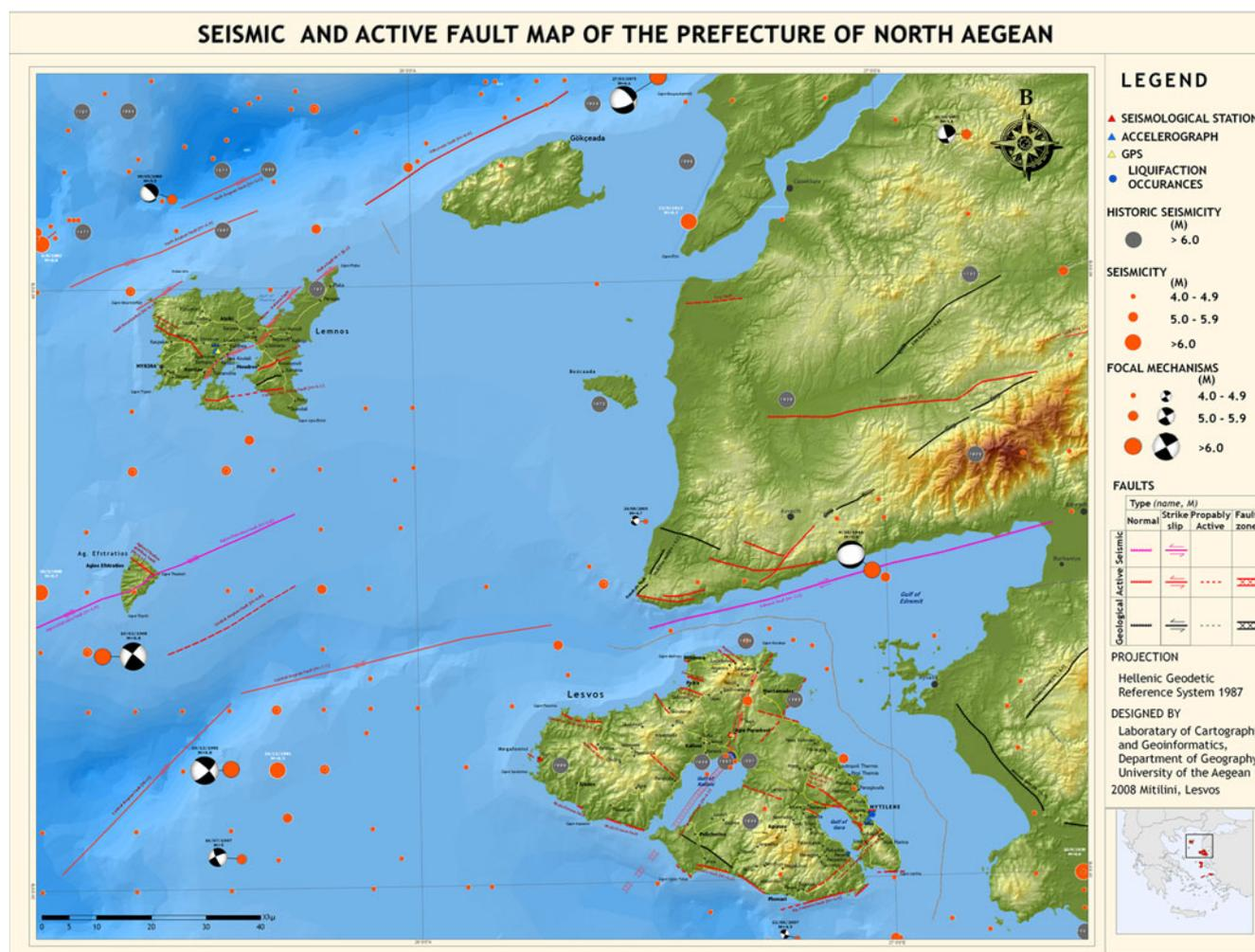
Fig. 4 Seismicity and active fault map of the North Aegean Region—north sheet (Zouros et al. 2008)
