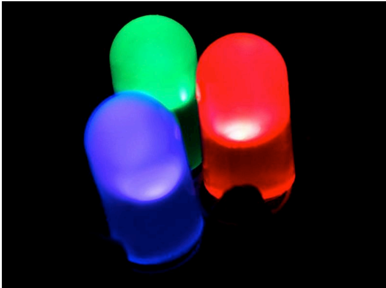
Close-up of red, green, and blue LEDs that form a single pixel in a large scale LED screen
