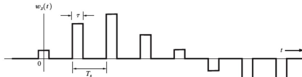
(c) Resulting PAM Signal (flat-top sampling, d = \tau/T_s = 1/3 )
