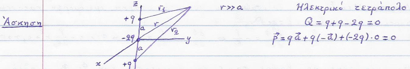
$$\phi = \frac{1}{4\pi\epsilon_0} \left( \frac{q}{r_1} - \frac{2q}{r} + \frac{q}{r_2} \right) = \frac{q}{4\pi\epsilon_0} \left( \frac{1}{r_1} - \frac{2}{r} + \frac{1}{r_2} \right)$$
