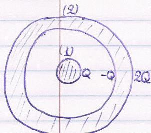
$$(1) 0 \leq r < R, \vec{E} = 0, \phi(r) = \phi(R) = \frac{Q}{4\pi\epsilon_0} \left( \frac{1}{R} - \frac{1}{R_1} + \frac{2}{R_2} \right)$$
