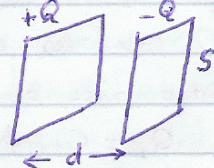
$$C = \frac{Q}{\phi} = \frac{\sigma S}{\phi} = \epsilon_0 \frac{S}{d}, \text{ π.χ. } C = 1F, d = 1mm \Rightarrow S = \frac{1F \times 10^{-3}}{10^{-11}} m^2 = 10^8 m^2 = 100 km^2$$
