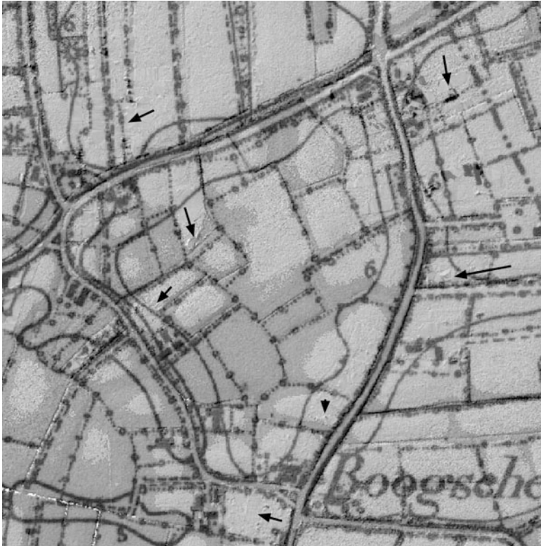
Fig. 10.7 LiDAR-GDEM overlaid with a historical topographical map of 1909. The LiDAR data have an average sampling density of 1 point/2 m 2 , resulting in an altimetric accuracy varying between 7 and 20 cm and a planimetric accuracy of 50 cm. The GDEM shows how fields are related to the micro-topography, revealing the artificial convex field topography resulting from digging drainage ditches at the borders and concentric ploughing. Artefacts from filtering out recent buildings are indicated by arrows (After Werbrouck et al. 2011, topographical background: historical Belgian topographical base map at scale 1:20,000, Dépot de la Guerre 1909, National Geographical Institute)
