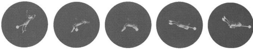
Fig. 2.8. The small sphere is the recovered camera position, and the line shows the view direction vector. The larger sphere, centered at the look-at point, gives an idea of the relative positioning of the recovered camera centers (see colour insert).
