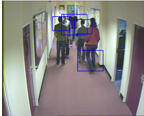
Fig. 2. This shows a frame in a sequence showing the main Torso detections. Note there are both true positive and false positive detections.
