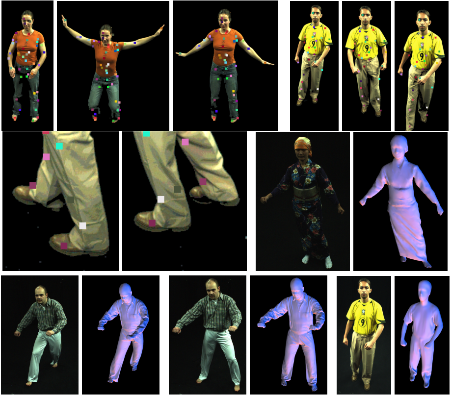
Fig. 4. (Upper row) Selected features tracked in three different frames for the yoga and walking sequences; (middle and lower row) two frames of the walking sequence in detail and side-by-side comparisons between input video frames and reconstructed poses for the human scan. Our framework correctly tracks 3D trajectories of features even in the presence of occlusions or appearance ambiguities. By combining the 3D point trajectories with our mesh deformation method, our algorithm is able to directly animate a human body scan.
