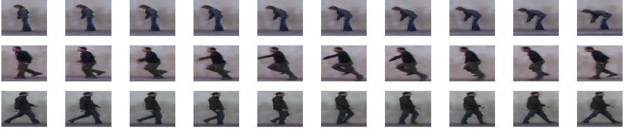
Fig. 4. Exemplary training sample sequences for extracting action primitives and building behavior histograms. The 40 \times 80 pixel detector window is centered around the human. The HOG-descriptors of all training images are used for clustering action primitives.
