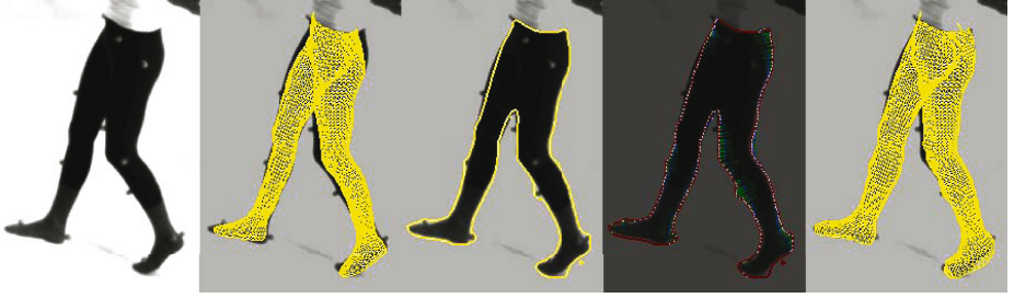
Fig. 4. Intermediate tracking results for one camera view. From Left to Right: Input picture, Reference model in current pose, Extracted Silhouette, 2D Correspondences (blue: ICP starting points, green: search path, white: 2D correspondence point), Final model adaptation.
