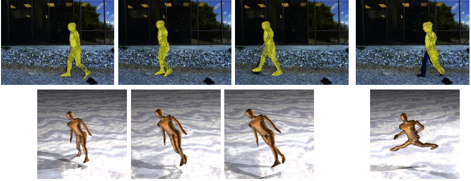
Fig. 4. Top row, from left to right: Tracking result for the sequence in Figure 3 but using the isotropic kernel density estimator. Results are not as good as in the anisotropic case. Rightmost: Without any motion prior, tracking fails already after a few frames. Bottom row: Synthesized view generated from the tracked pose.
