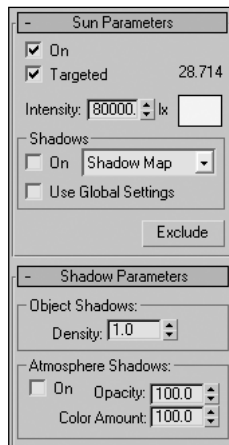
Figure 11-11. The Sun Parameters and Shadow Parameters rollouts
