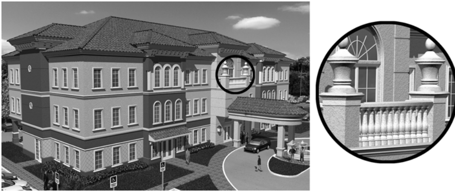
Figure 17-3. Using the Instance command to reduce file size
