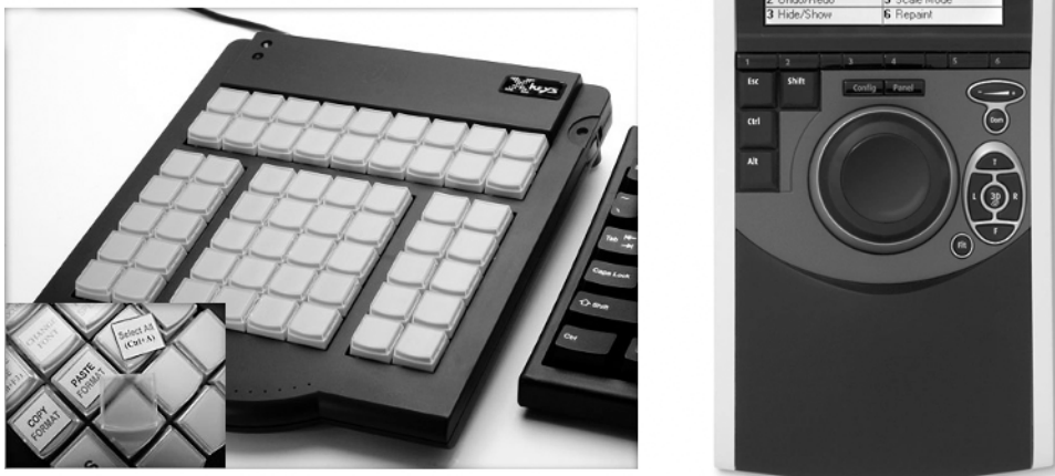
Figure B-3. The keypad (left) and 3D motion controller (right)
