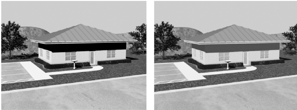
Figure 12-1. Direct illumination (left) and global illumination (right)
