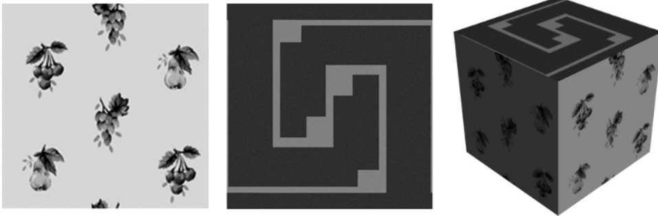
Figure 9-8. Two different maps of a multi/sub-object material applied to the same object (using map channels)
