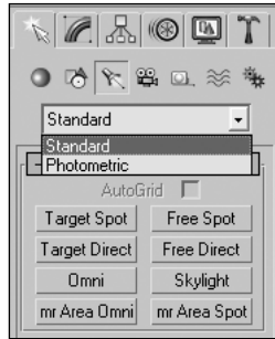
Figure 10-1. The two light types: standard and photometric
