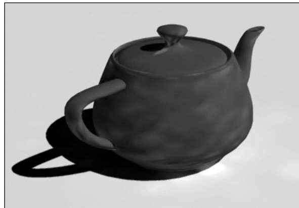
Figure 12-6. Radiosity imperfections in the illumination of an object
