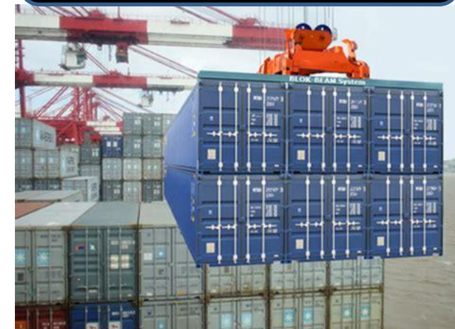
'Blok beam' system (6 empty FEU)
