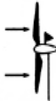
Upwind with active powered steering switched by wind vane
