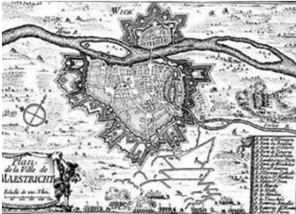
Fig. 2. Siege of Maastricht in 1673 by King Louis XIV. Vauban, in charge of the operation, introduced the parallel trench strategy, with zigzag approaches and three parallels.
