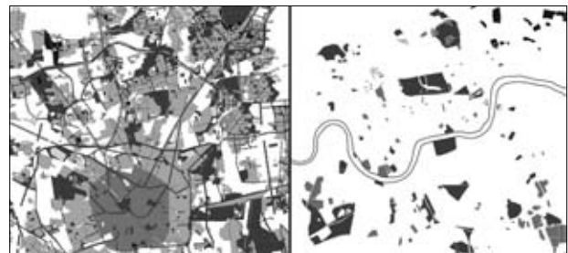
Fig. 1, Level of detail obtained in the same amount of time using CAD (left) and GIS (right) tools. Graphics at the same scale. Piano Intercomunale Milanese, 1961-65; London City Plan, 1943.
