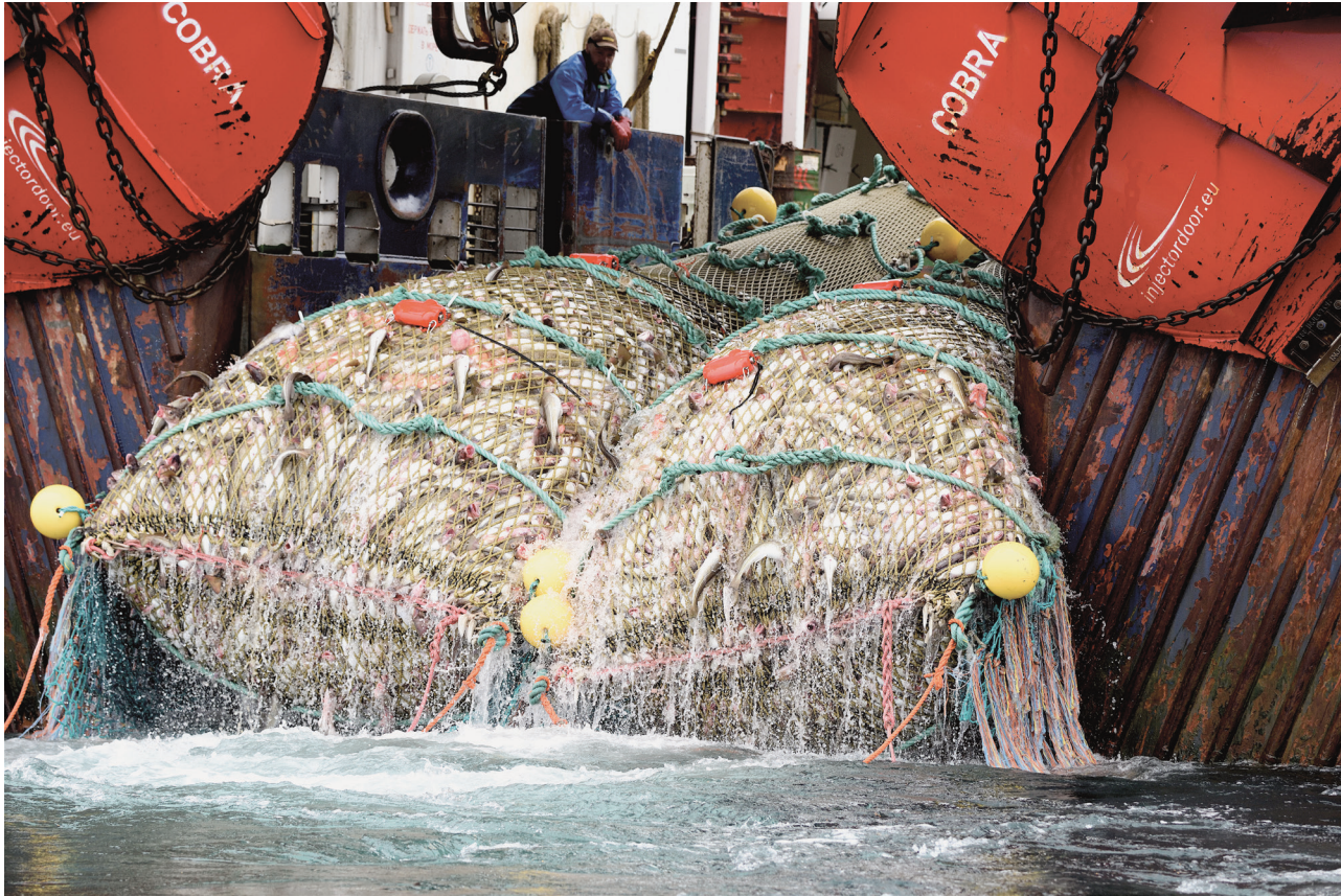
FIG. 21.15 A bottom trawl net of cod being loaded onto a fishing ship near Svalbard, Norway, July 2016. Black steel otter boards that hold the net open as the trawling net moves along the sea bed are visible. (Photograph by Carl Safina)
