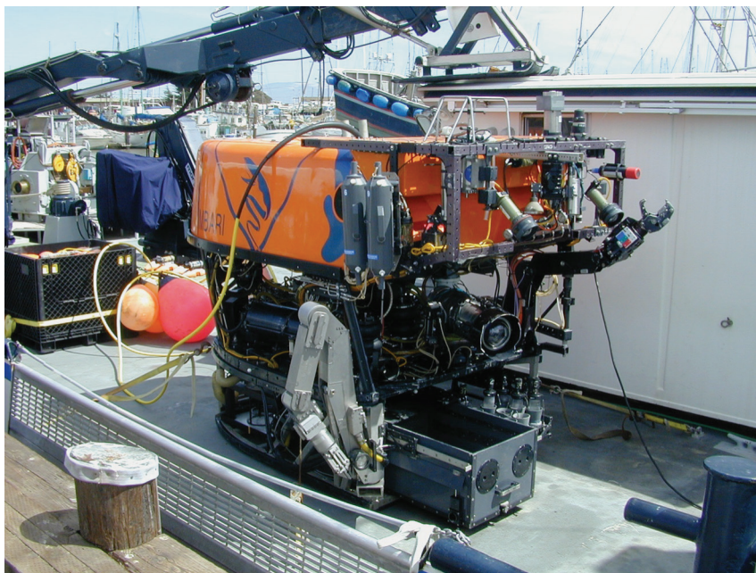
FIG. 1.7 The Ventana , an ROV operated by the Monterey Bay Aquarium Research Institute in central California. The vehicle is connected to the mother vessel by a cable and is equipped with high-definition video, two grabber arms, and a variety of samplers, including a sample box that can be seen in the front. Newer versions have been launched. (Photograph by Jeffrey Levinton)
