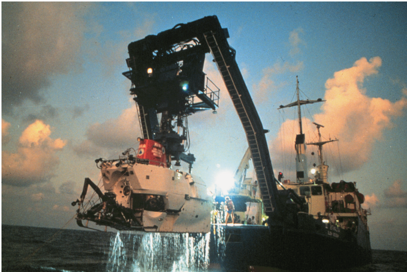
FIG. 1.6 The Alvin , a submarine capable of diving to 4,500 m, is equipped with accurate navigation and photography equipment and underwater manipulators. The Alvin is the great workhorse of the world research submarine fleet and is scheduled to be replaced in the coming years. (Photograph courtesy of Richard Lutz)
