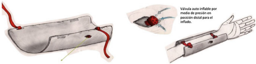
Fig. 2 Design proposal: pneumatic splint for oxygen delivery to extremities by group no 5 (Source Hananias et al. 2016 [27])
