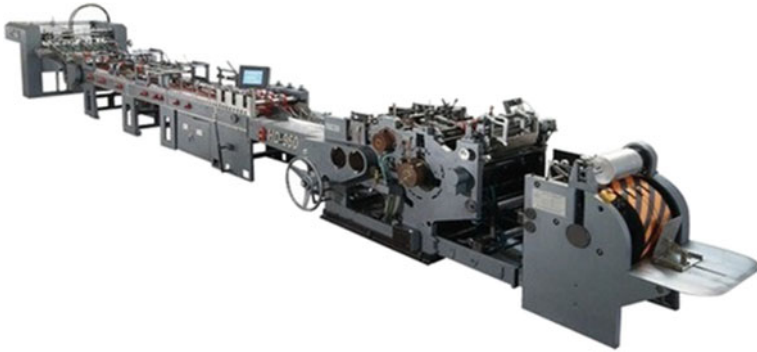
Fig. 3 Existing paper carry bag making machine: expensive, bulky and labour intensive (Source http://www.tradeindia.com )
