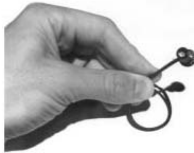
Figure 1. Ultrasonic microphone element for position tracking system. (Beltpack transmitter not shown.)
