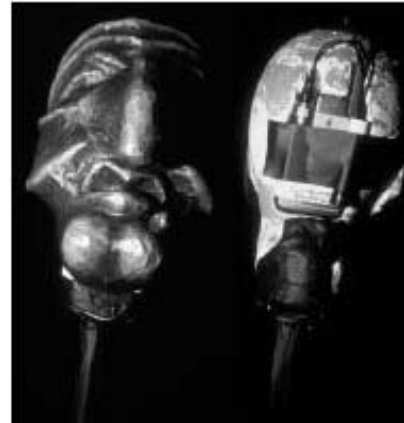
Figure 8. Detail of foam head on witch staff, showing embedded tracking device.
