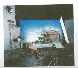
The lighting set-up for an outdoor shot in A Close Shave. For this shot the key light (I) assumes the sun position. The shadows are filled by 'bouncing' a narrowbeamed lamp (4) off the large white fill board (6). Three back lights (2,3,5) are used to give emphasis to certain parts of the set, such as the cabin of the truck and details on the rooftop. When positioning these, care is needed not to create secondary shadows from the camera's viewpoint (7).
